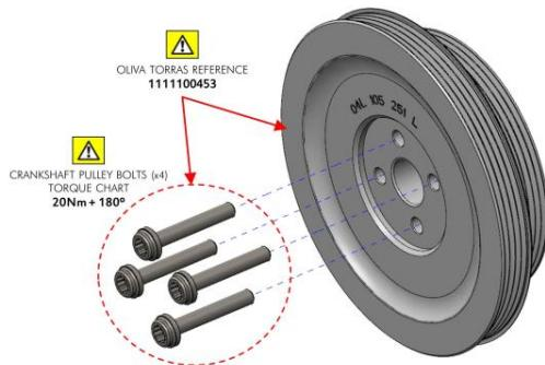
As a result of an agreement with VW, Oliva Torras is in a position to supply this pulley, as an option, with the Drive kit, reference **1111100453**. New bolts are also included, as recommended by the bodybuilder, once the crankshaft pulley is replaced.
